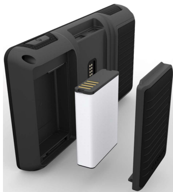
Unit Overview - Battery
